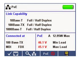
The Net Prowler has a really useful feature to test PoE for IP cameras, where you can connect your IP camera's network cable to your Prowler, and actually
