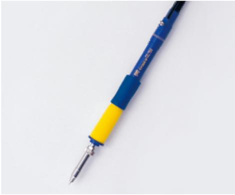
Hakko FM-2026 N<sub>2</sub> gas Soldering Iron, ceramic heater in the FM-2026 handpiece preheats Nitrogen gas, improving efficiency and reducing the amount of oxygen in the solder connection area (less oxidation), Uses T-15 tips.
