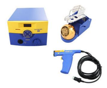
Hakko FM-205 Digital Desoldering Tool uses compressed air to generate a vacuum rather than an internal pump. Providing higher vacuum pressure, increased suction flow, and a lower station cost.
