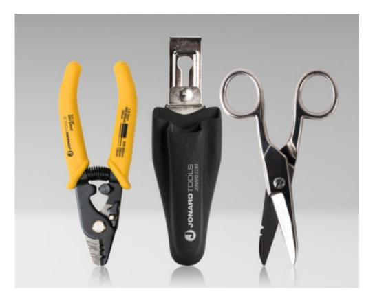
Includes the JIC-375 Fiber Optic Stripper, ES-1964 Electrician's Scissor, and molded plastic pouch with metal clip.
